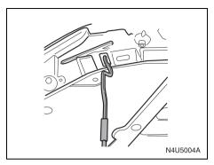
3) Lift the hood, release the hood prop from its retainer and place the hood prop into the slot in the hood.
